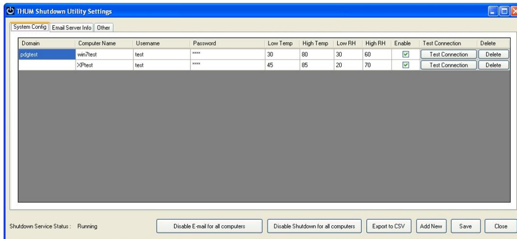
THUM Shutdown is a utility to shutdown multiple Windows computers based on the readings received from a locally installed THUM(Temperature Humidity USB Monitor) device. This is an add-on to the THUM software.
